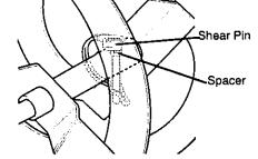
To replace a broken shear bolt, proceed as follows:
